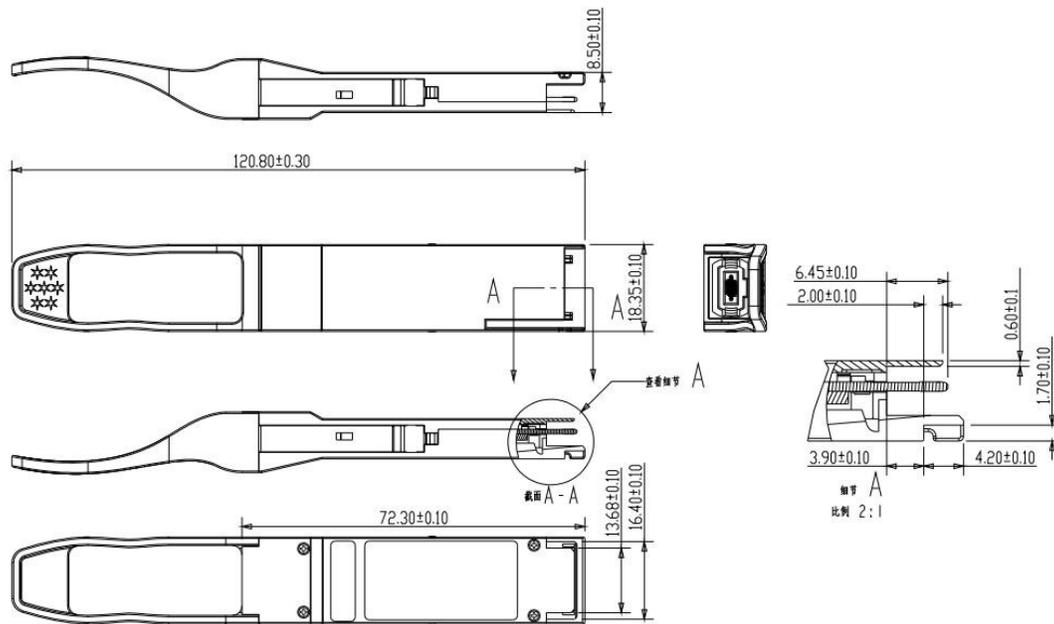
**Figure 13. Mechanical Specifications**
