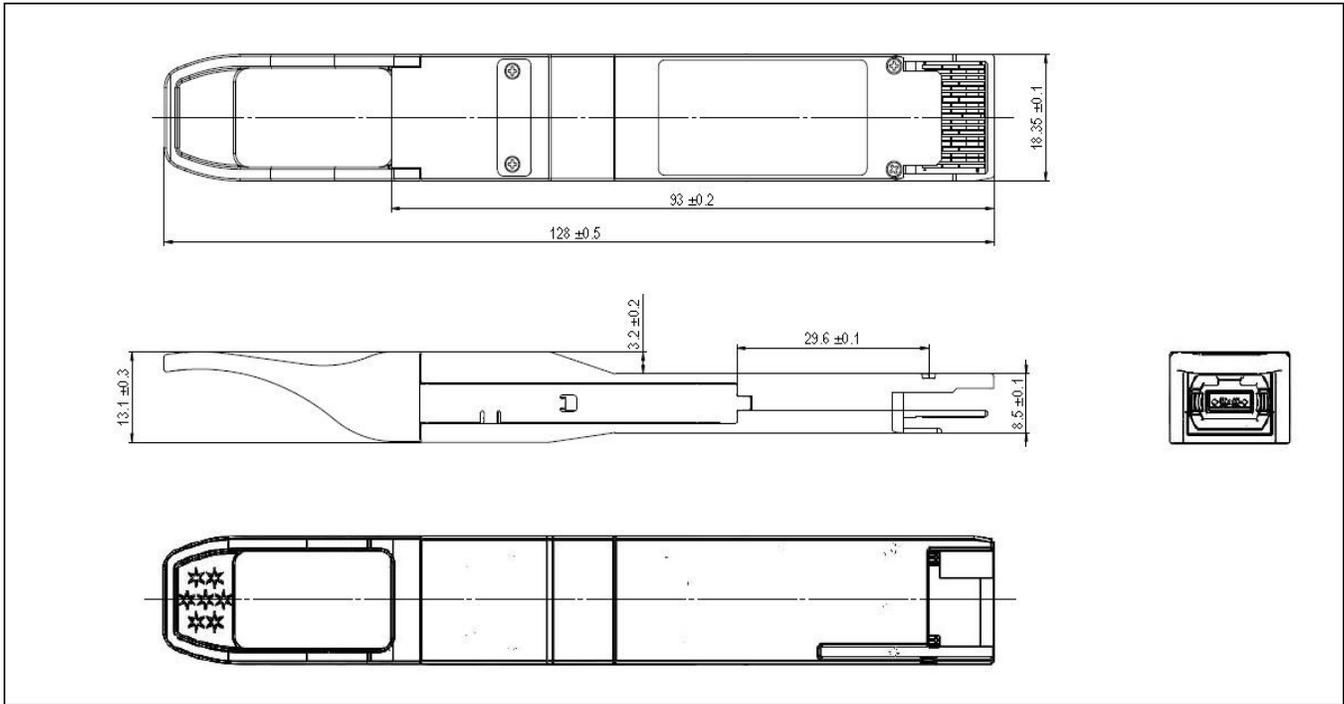
Figure10. Mechanical Specifications
